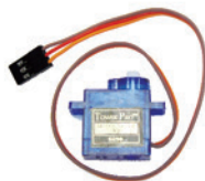
SG90伺服電動機 (360度連續轉動) / SG90 Servo Motor (360-degree Continuous Rotation)
